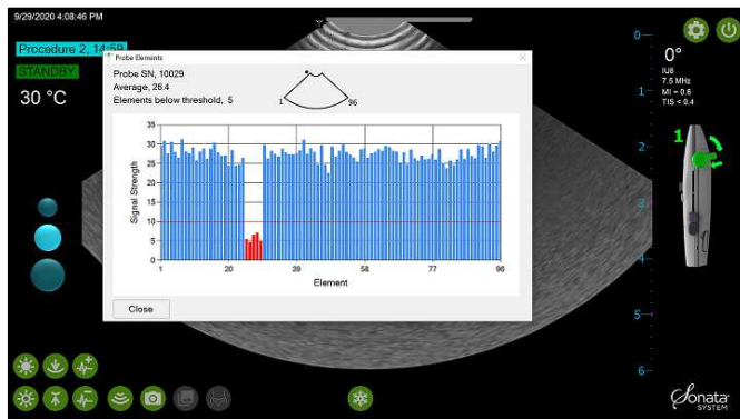
Figure 6-20. Transducer Element Check.
