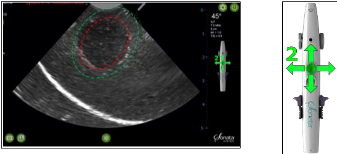
Figure 4-12. Use SMART Control to adjust the ablation depth and size.
