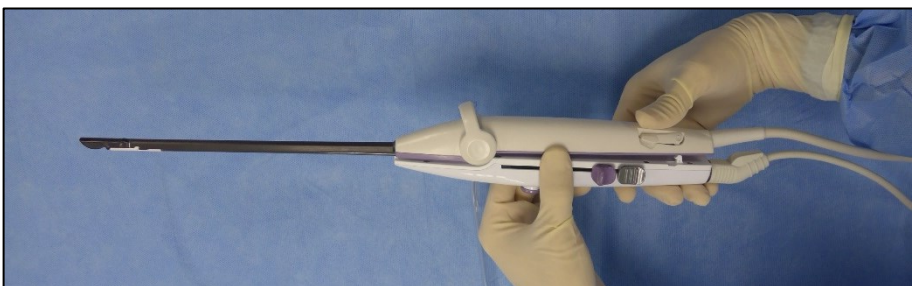
Figure 3-16. Snap the handles together while keeping the IUUS Probe Tip and the RFA Handpiece Tip connected.
