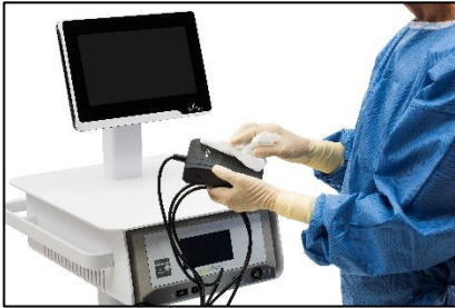
Figure 5-12. Clean parts and external surfaces with a medical grade low alcohol disinfectant.
