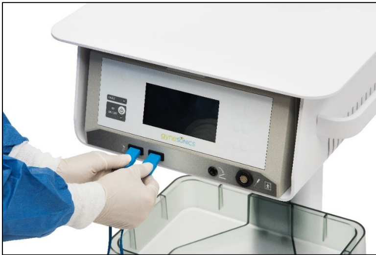
Figure 3-13. Connect both Dispersive Electrode cables to the front of the RF Generator.
