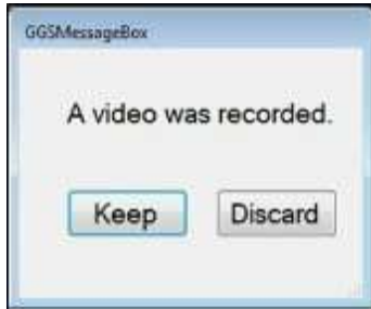
Figure 5-5. Video “Keep” or “Discard” window will be displayed when IUUS Probe it disconnected.
