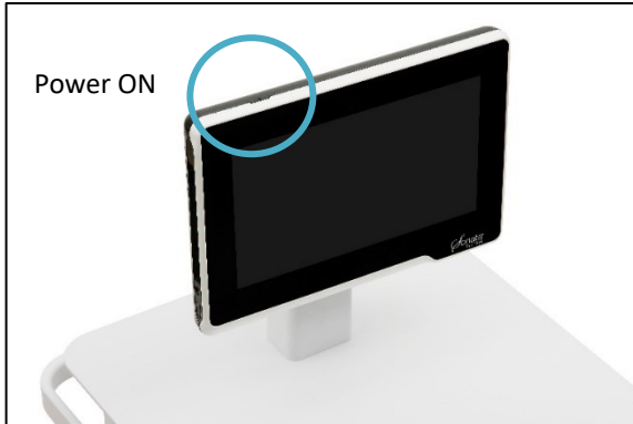
Figure 3-6. Power ON by pressing the power button on upper-left corner of SMART Tablet.
